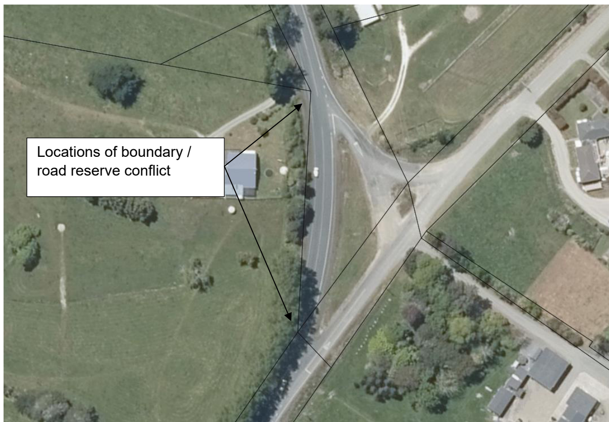
Figure 6-2: Existing boundary locations
